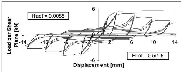
Figure 10 – E<sub>SH</sub> Calculated Hysteresis Curve (Calculated Monotonic Curve Shown in Grey)
