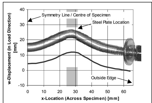
Figure 9 – Deformed F\_SHT Dowel Shape Comparison (Calculated Shape in Black)
