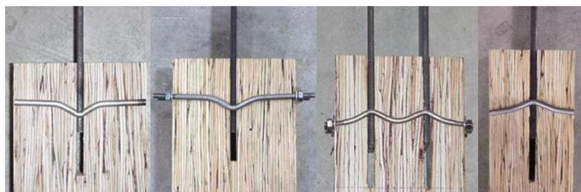
Figure 3 – Deformed Fasteners (Series D, E, F and G)
