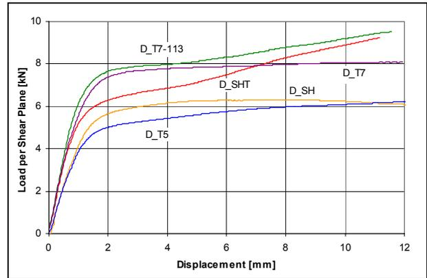
Figure 4 – Average Load-Displacement Curves for Series D Monotonic Tests
