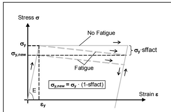
Figure 7 – Wood/Steel Plate Material Behavior
