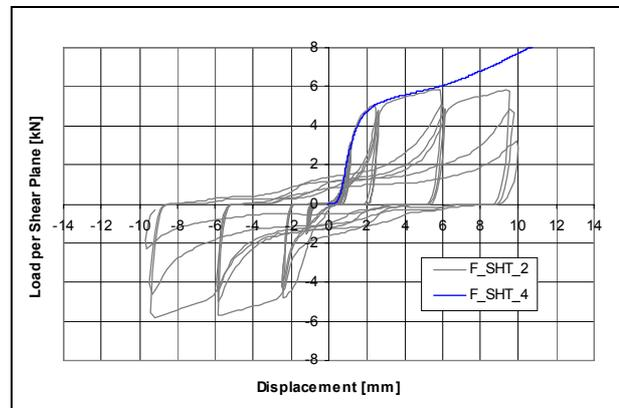
Figure 5 – Typical  $F_{SH}$  and  $F_{SHT}$  Cyclic and Monotonic Load-Displacement Curves
